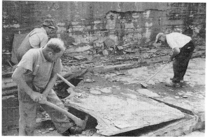
Fig.2. Quarrying the shale by hand with the Reuthaue (slate mattock) after loosening by blasting. Quarry of J. Fischer, Ohmden, 1968.
