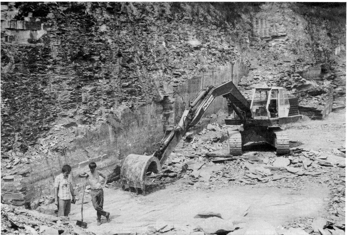
Fig.3. The Upper and Middle Epsilon in the quarry of J. Fischer, Zell, 1976. The excavator is removing this overburden.
