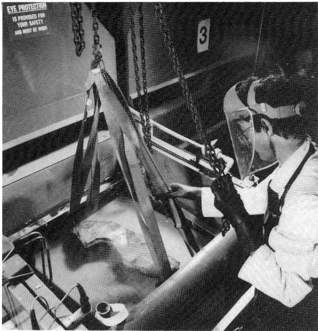
Fig.2. The initial acid immersion of the specimen shown in Fig.1.
