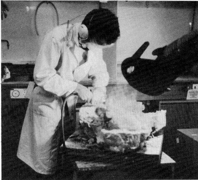
Fig.1. Mobile local exhaust ventilation system used for the removal of dust during mechanical preparation. Palaeontology Laboratory, British Museum (Natural History). (Courtesy of S. Rowles).
