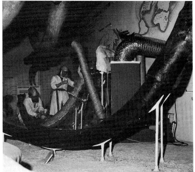
Fig.2. Portable fume extraction equipment used to exhaust styrene from gallery area during work with polyester resin. Fossil Mammal Gallery, British Museum (Natural History).
