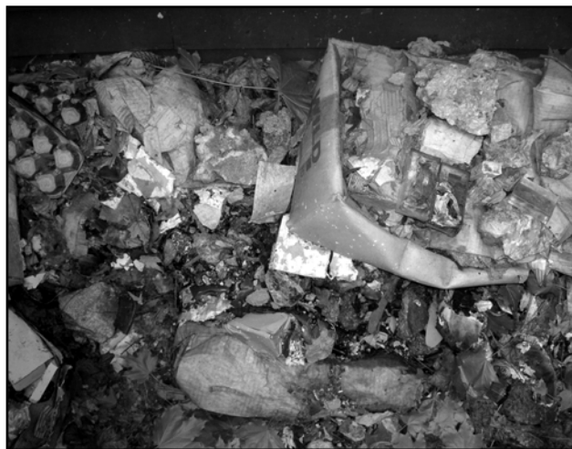
Figure 7. Close-up of debris from the workroom. Melted plastic flower pots, melted 35-mm transparencies, cardboard, and newspaper formed a matrix for mineral specimens. Immediately after the fire, all this was black.
