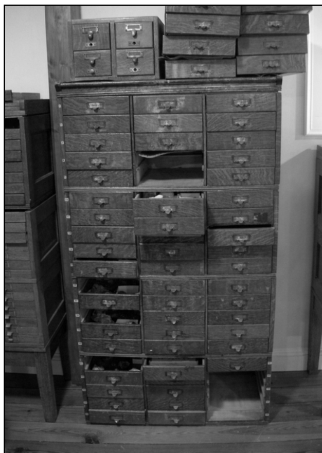
Figure 9. An historic mineral cabinet, sequentially owned by Dr. Leonard G. Berry and Dr. George W. Robinson before I acquired it, did not survive the deleterious effects of the water associated with fighting the fire. This picture was taken seven months after the fire. The cabinet had dried and the drawers were no longer frozen, but many of them would not open because the drawer bottoms buckled downward when they swelled as can be seen in the middle of the cabinet. To get the mineral specimens out of this cabinet, I had to disassemble it piece by piece. Note the walls and floor are now like new.
