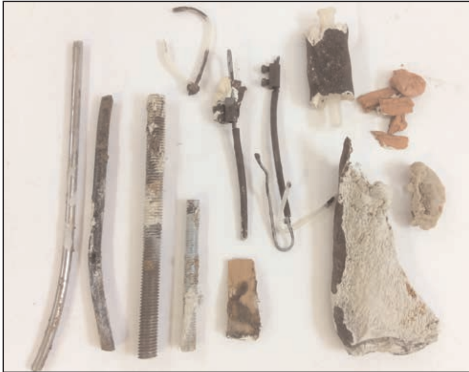
Figure 2. A selection of materials applied during previous restoration treatments found and removed from the specimen.
