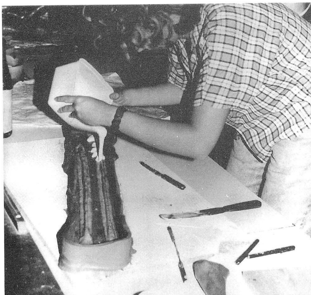
Figure 5. Silicone rubber is being poured over the embedded premodels.
