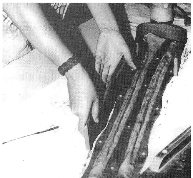
Figure 4. "Keyholes" have been made in the clay bed, and a clay wall is being fitted.
