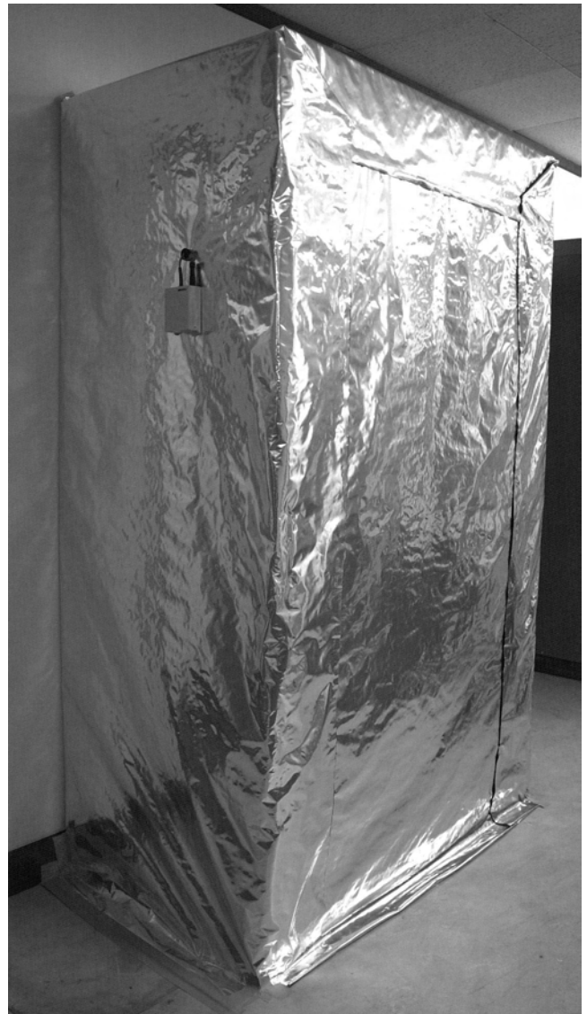
Figure 9. The completed wrapped cabinet with the door flaps sealed.
