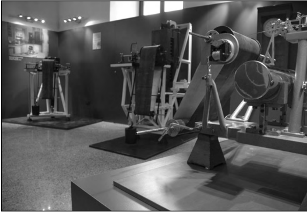
Figure 7. The room of the seismologic instruments, on the left the two mechanical Wiechert's seismographs with, on the right, the Ishimoto seismograph.
