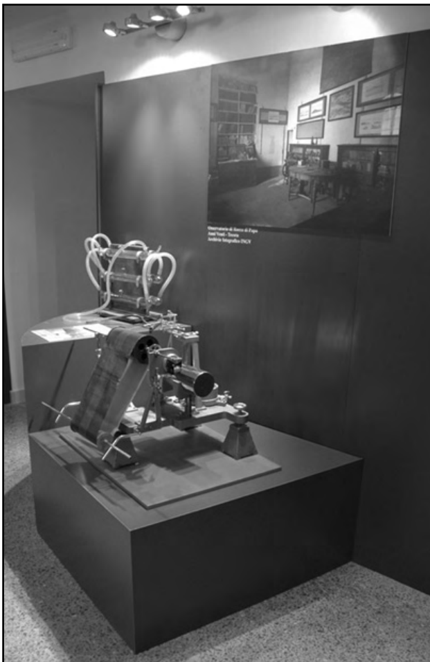
Figure 8. The Ishimoto seismograph, recorded one of the two horizontal components of ground motion, amplifying motions by a factor of 100. In the background, the instrument used to blacken the paper with the smoke, as the ancient seismographs used smoked paper to record the seismic signals.
