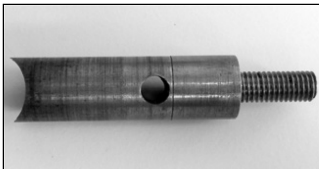
Figure 8. A 7 mm tightening hole drilled into the finished cutting bit.
