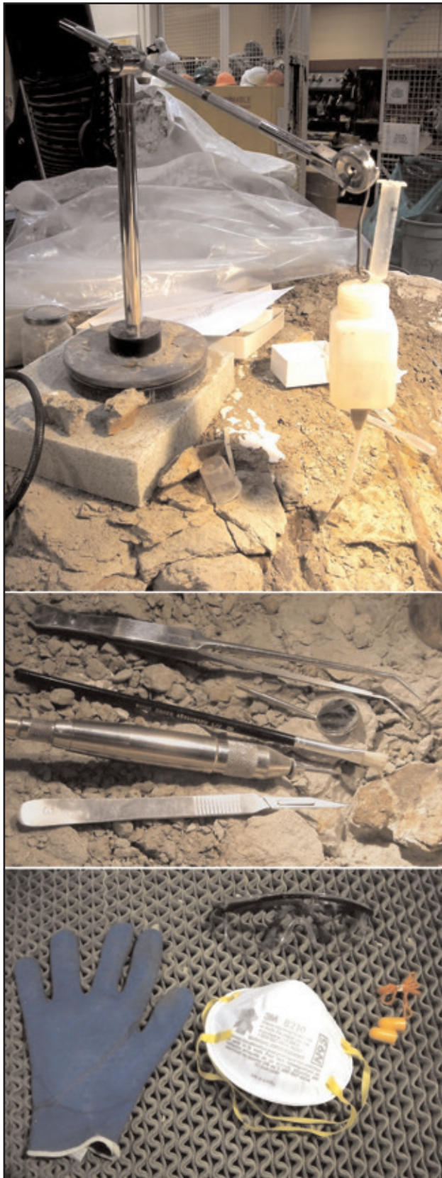
Figure 2. Selected photographs by D.H.T. illustrating selected tools and their use during preparation. Top: a home-made system to drip consolidating glue into a crack in the bone, Middle: various hand tools for detailed work on the material including a dental pick and mirror. Bottom: safety equipment - anti-vibration gloves, ear defenders (ear plugs), goggles and mask, all on a rubber mat. All of these images were first published on the Archosaur Musings.
